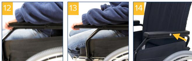
**The spring button must lock back into position after adjustment. Select the closest position, if necessary.**
